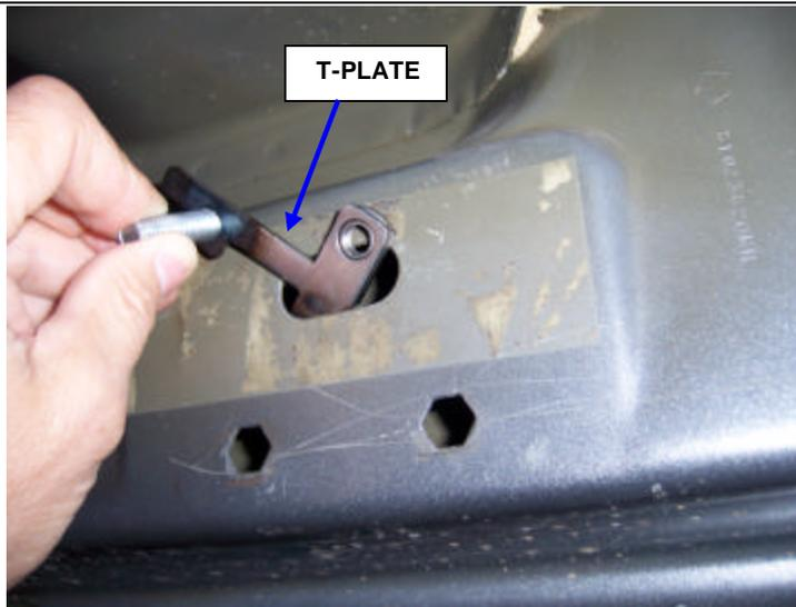
**STEP 2.** INSERT (1) OF THE T-PLATES THROUGH THE OBLONG HOLE IN THE BODY PANEL AND POSITION THE PLATE INSIDE THE PANEL AS SHOWN. PLACE (1) OF VINYL GASKETS TO THE T-PLATE.
