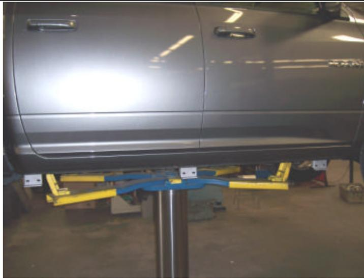
**STEP 4.** REPEAT THE ABOVE PROCEDURE TO INSTALL THE CENTER AND REAR MOUNTING BRACKETS.
