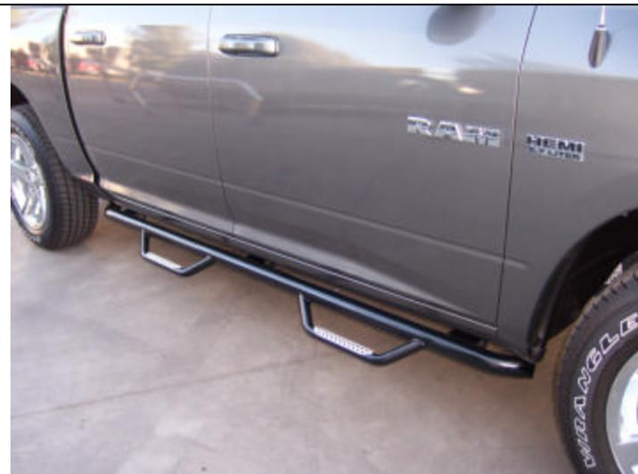
**STEP 6.** ALIGN THE SIDE STEP WITH THE VEHICLE AND TIGHTEN ALL MOUNTING BRACKET AND SIDE STEP NUTS AND BOLTS. REPEAT THE ABOVE PROCEDURE TO INSTALL THE DRIVER SIDE BRACKETS AND SIDE STEP.
