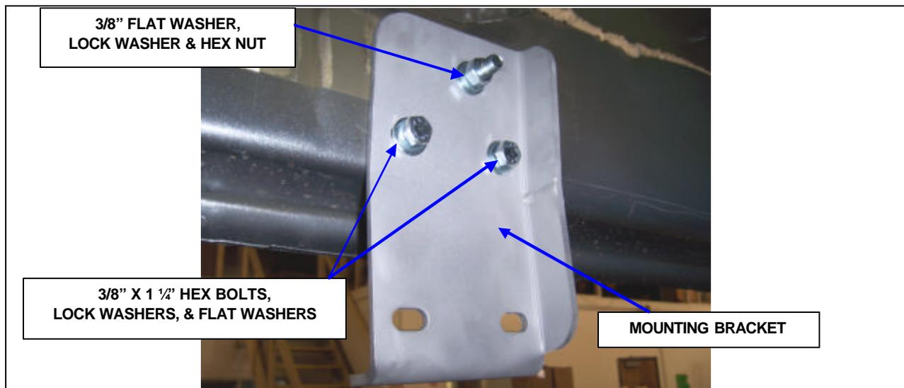
**STEP 3.** ATTACH ONE OF THE MOUNTING BRACKETS TO THE BODY PANEL USING THE T-PLATE (2) 3/8" X 1 1/4" HEX BOLTS, (3) 3/8" FLAT WASHERS, (3) 3/8" LOCK WASHERS AND (1) 3/8" HEX NUT. HAND TIGHTEN.
