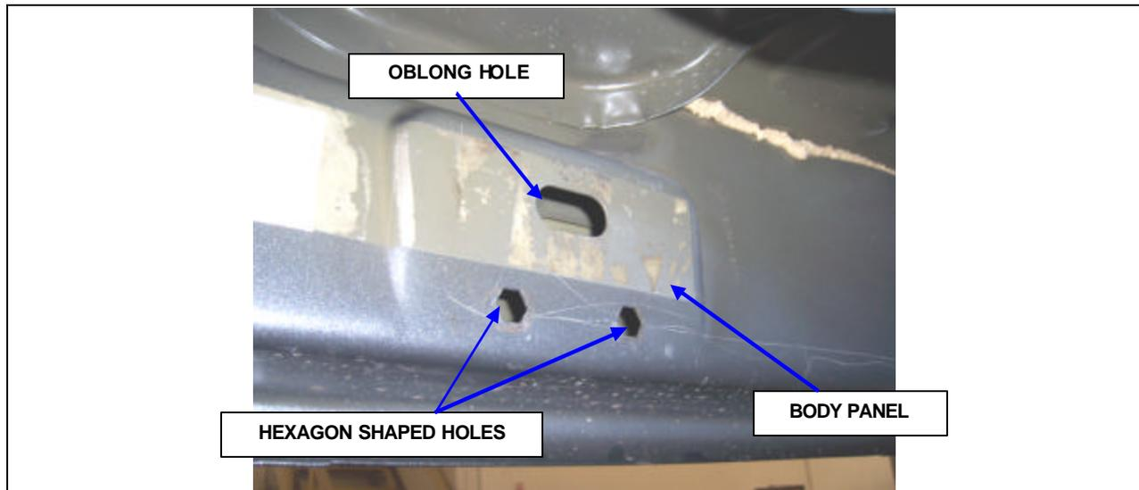
**STEP 1.** THIS INSTALLATION USES (3) MOUNTING BRACKETS PER SIDE. BEGIN BY INSTALLING THE PASSENGER SIDE FRONT BRACKET. LOCATE THE (2) HEXAGON SHAPED HOLES IN THE UNDERSIDE OF THE BODY PANEL AT THE FRONT OF THE CAB AND REMOVE THE TAPE COVERING THE OBLONG HOLE.
