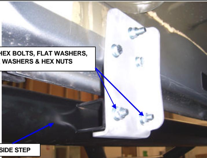
**STEP 5.** ATTACH THE PASSENGER SIDE STEP TO THE MOUNTING BRACKETS USING (2) 3/8" X 1 1/4" HEX BOLTS, (4) FLAT WASHERS, (2) LOCK WASHERS AND (2) HEX NUTS FOR EACH BRACKET.
