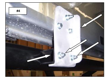
**STEP-4** ALIGN THE SIDE STEP WITH THE VEHICLE AND TIGHTEN ALL MOUNTING BRACKET AND SIDE STEP NUTS AND BOLTS. **REPEAT THE ABOVE PROCESS TO INSTALL THE DRIVER SIDE BRACKETS AND SIDE STEP.**
