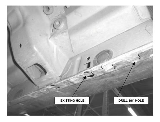
**STEP 5.** Locate the hole in the lower body pinch mold for the center-mounting bracket. The center bracket requires drilling an additional mounting hole. Measure rearward from the center of the existing hole approximately 3 3/4" and drill a 3/8" hole in the body pinch mold hole.
