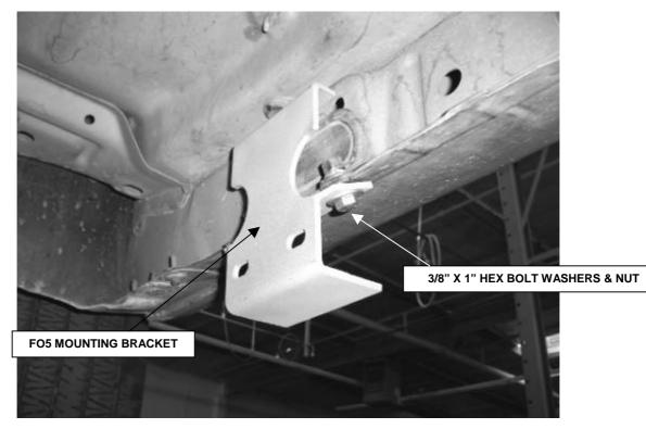
**STEP 4.** Loosely attach the flange of the front mounting bracket to the bottom of the lower body pinch mold using the 3/8" x 1" hex bolts, washers, and nuts as shown.
