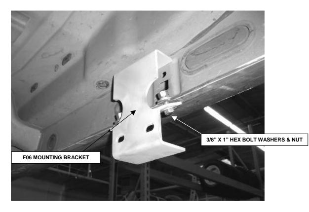
**STEP 8.** Loosely attach the flange of the mounting bracket to the bottom of the lower body pinch mold using the 3/8" x 1" hex bolts, washers, and nuts.
