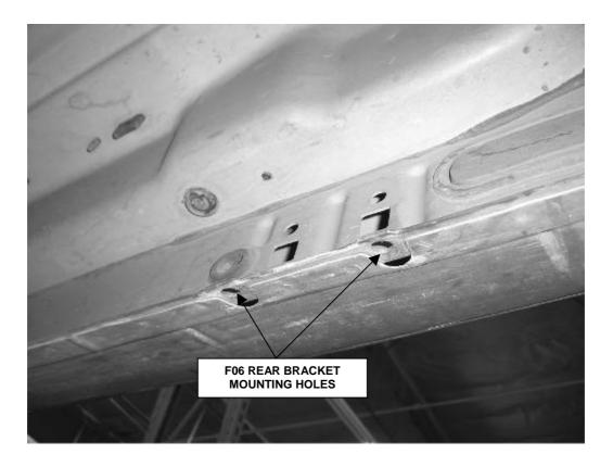
STEP 7. Locate the holes in the lower body pinch mold for the rear-mounting bracket.
