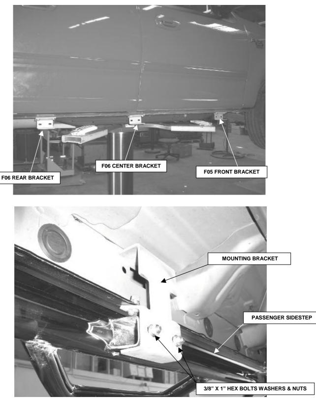
**STEP 9.** Position the passenger sidestep up to the mounting brackets and loosely attach it to the brackets using the 3/8" x 1" hex bolts, washers and nuts as shown.
