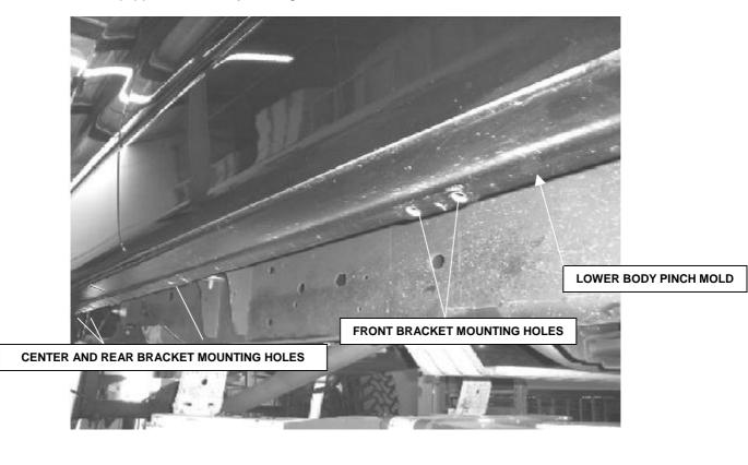
STEP 2. This installation uses three mounting brackets per side.
