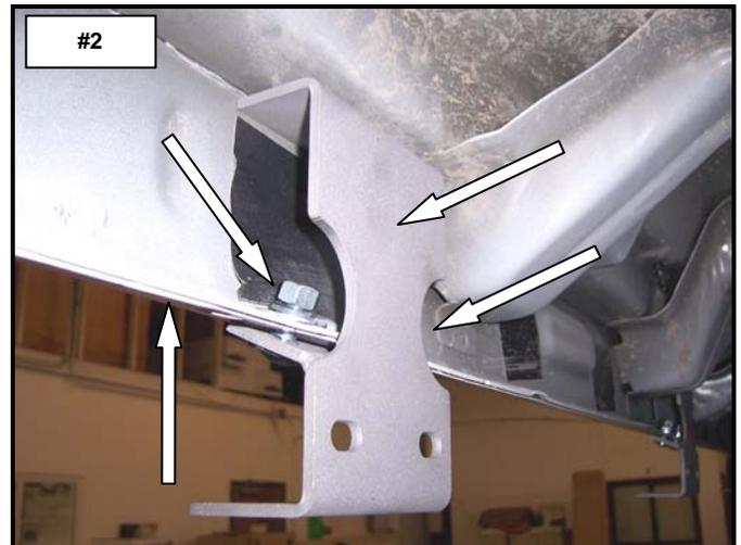
**STEP 2.** ATTACH EACH OF THE MOUNTING BRACKETS TO THE PINCH MOLD USING (2) 3/8" X 1" CARRIAGE BOLTS, (2) FLAT WASHERS, (2) LOCK WASHER AND (2) HEX NUTS. HAND TIGHTEN. **PHOTO'S #2 & #3**
