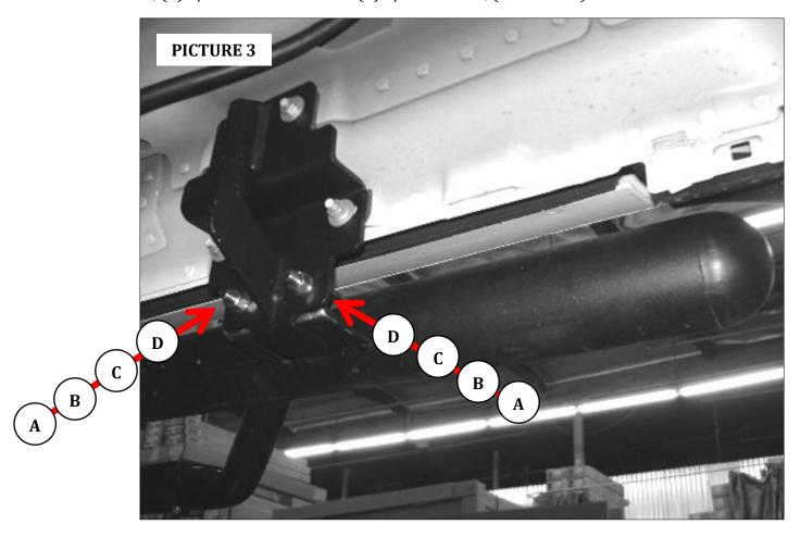
**Step-5** Align the side step with the vehicle and tighten all bracket and side step nuts and bolts,. Repeat the above steps to install the passenger side brackets and side step. Remember to check and retighten the nuts and bolts every six months.
