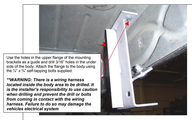
**Step 4**. Loosely attach the lower flange of the mounting brackets to the bottom of the body pinch mold using the 3/8" x 1" carriage bolts, flat washers, lock washers and nuts as shown.
