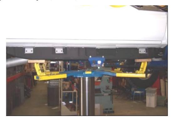
**Step 5.** Position the passenger sidestep up to the mounting brackets and loosely attach it to the brackets using the 3/8" x 1 1/4" hex bolts, flat washers, lock washers and nuts.
