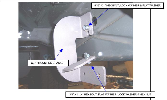
**STEP 4.** Loosely attach one of the C07P mounting brackets to the rocker panel and pinch mold using the 5/16" and 3/8" fasteners as shown.
