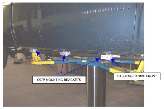
**STEP 5**. Locate the holes in the body for the center and rear mounting brackets. Measure rearward from the front fender bolt 37 3/4" for the center and 67" for the rear bracket. Repeat steps 3 & 4 to install the center and rear brackets.
