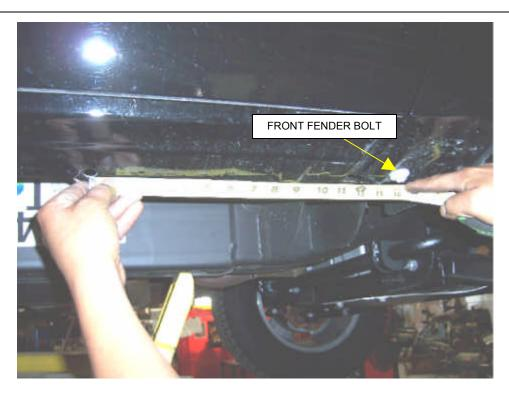
**STEP 2.** This installation uses three mounting brackets per side. Begin by installing the passenger side front mounting bracket. Measure reward from the front fender bolt approximately 14" and locate the holes in the body pinch mold, rocker panel and the plastic plug in the rocker panel.
