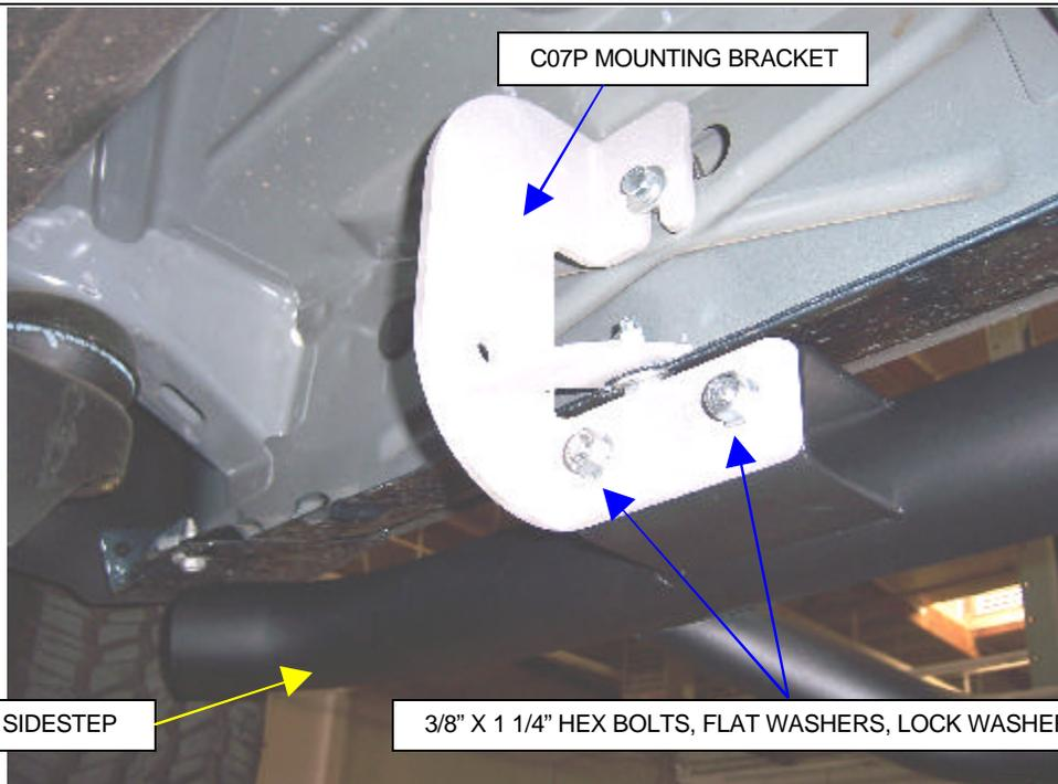
**STEP-6** Position the passenger sidestep up to the vehicle and loosely attach it to the mounting brackets using the 3/8" x 1 1/4" hex bolts, flat washers, lock washers and hex nuts.
