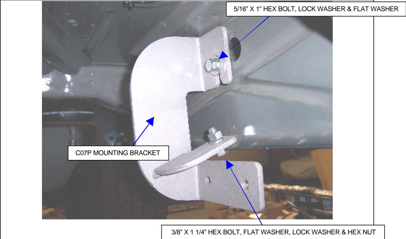
**STEP-4** Loosely attach one of the C07P mounting brackets to the rocker panel and pinch mold using the 5/16" and 3/8" fasteners as shown.
