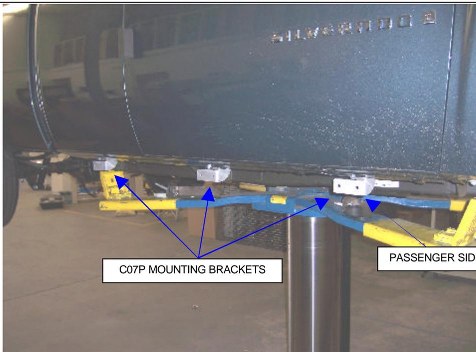
**STEP-5** Locate the holes in the body for the center and rear mounting brackets. Measure rearward from the front fender bolt 37 3/4" for the center and 67" for the rear bracket. Repeat steps 3 & 4 to install the center and rear brackets.
