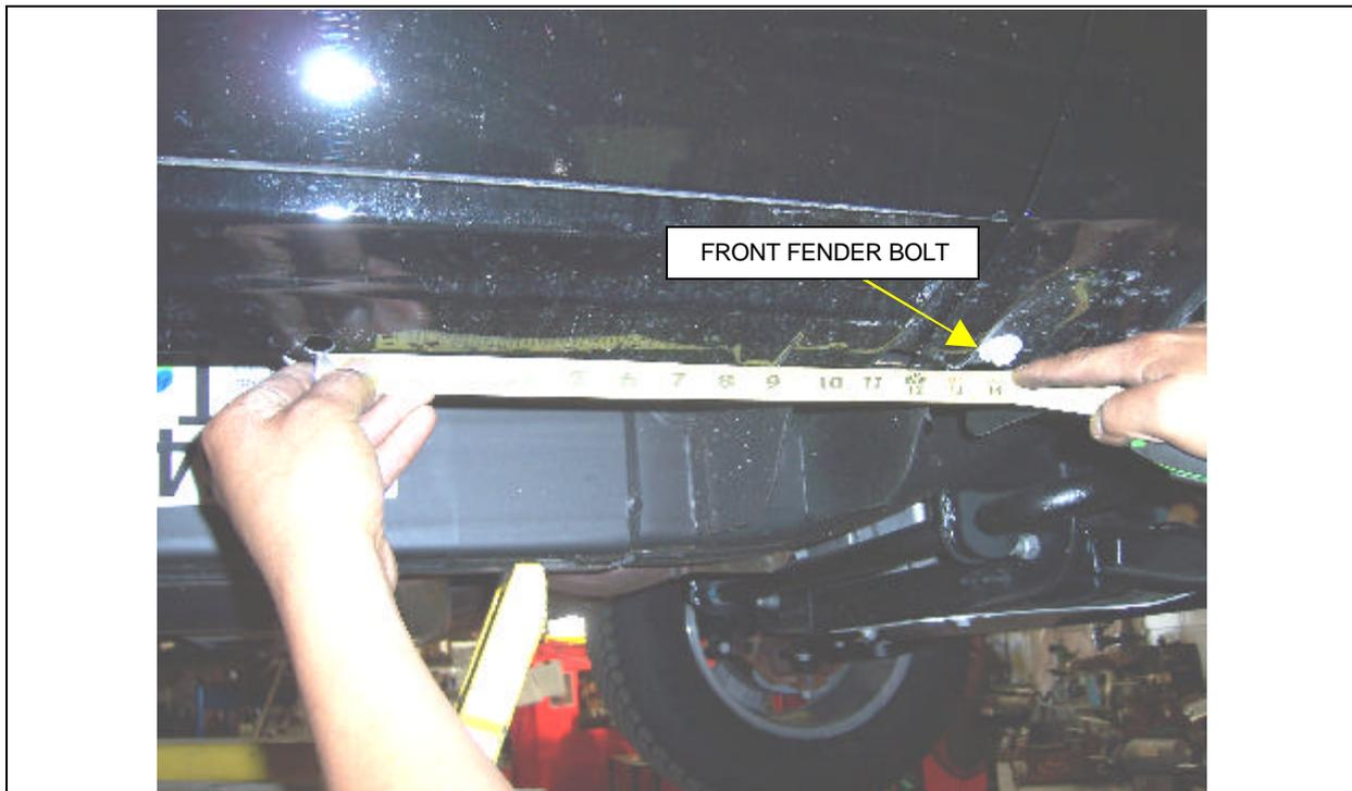
**STEP-2** This installation uses three mounting brackets per side. Begin by installing the passenger side front mounting bracket. Measure rearward from the front fender bolt approximately 14" and locate the holes in the body pinch mold, rocker panel and the plastic plug in the rocker panel.
