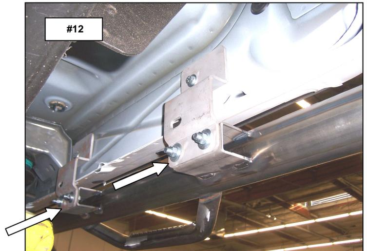
**Step-8** Align the side step with the vehicle and tighten all nuts and bolts.
