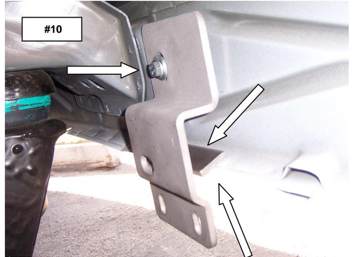
**Step-6** Passenger side rear bracket installation.
