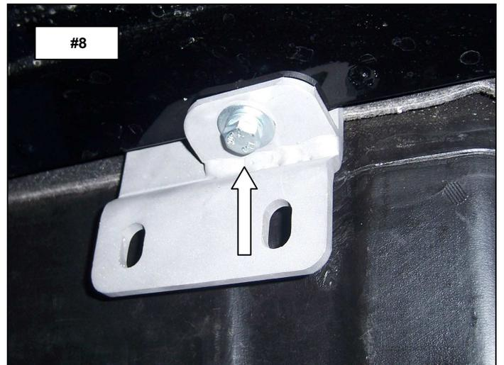
**Step-5** Passenger side Center bracket installation.
