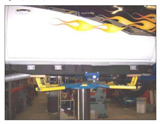
**STEP-5** Position the passenger sidestep up to the mounting brackets and loosely attach it to the brackets using the 3/8" x 1 1/4" hex bolts, flat washers, lock washers and nuts.
