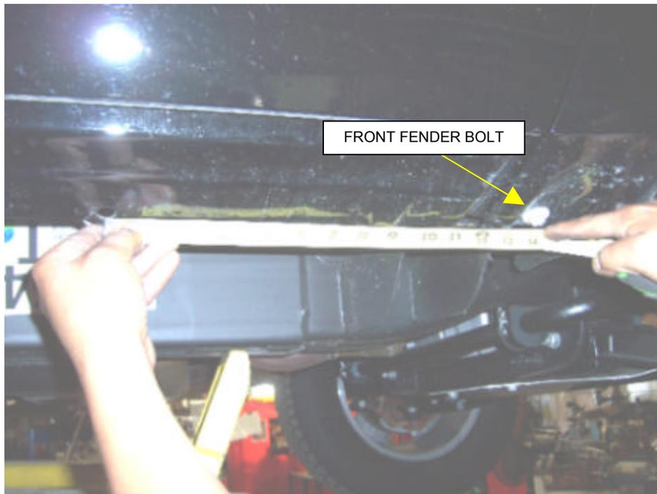
**STEP 2.** This installation uses three mounting brackets per side. Begin by installing the passenger side front mounting bracket. Measure rearward from the front fender bolt approximately 14" and locate the single hole in the body pinch mold and the square nut spot welded in the rocker panel.
