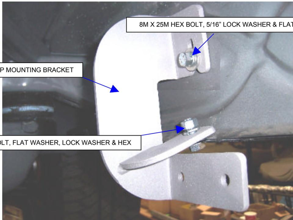
**STEP 3.** Loosely attach one of the C07P mounting brackets to the rocker panel and pinch mold using the 8M, 5/16" and 3/8" fasteners as shown.
