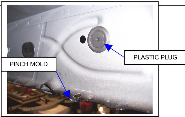
**STEP 4.** Locate the holes in the body pinch mold and rocker panel for the center and rear mounting brackets. Measure rearward from the front fender bolt approximately 58 7/8" for the center and 75 1/8" for the rear bracket. Remove the plastic plugs from the rocker panel and install 5/16" U-NUTS in the rocker panel as shown.
