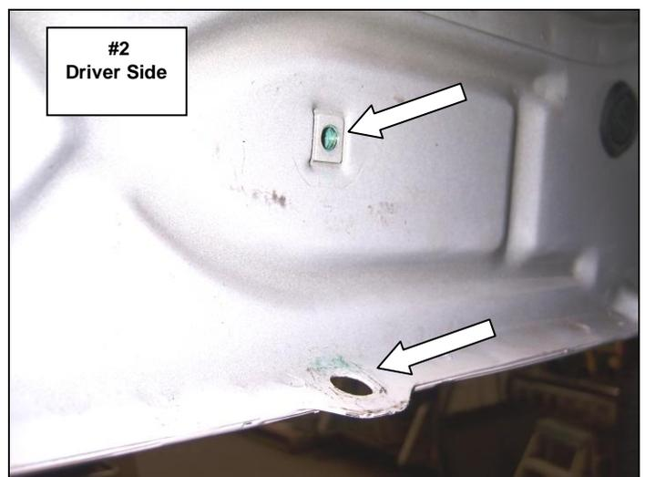
**Step-2** Attach one of the driver side brackets to the pinch mold using (1) M8 hex bolt, (2) 5/16" flat washers, (1) 5/16" lock washer and (1) M8 hex nut, and to the rocker panel using (1) M8 hex bolt, (1) 5/16" lock washer and (1) 5/16" flat washer. Leave the nut and bolts loose for final adjustment, **(Photo 3)**.
