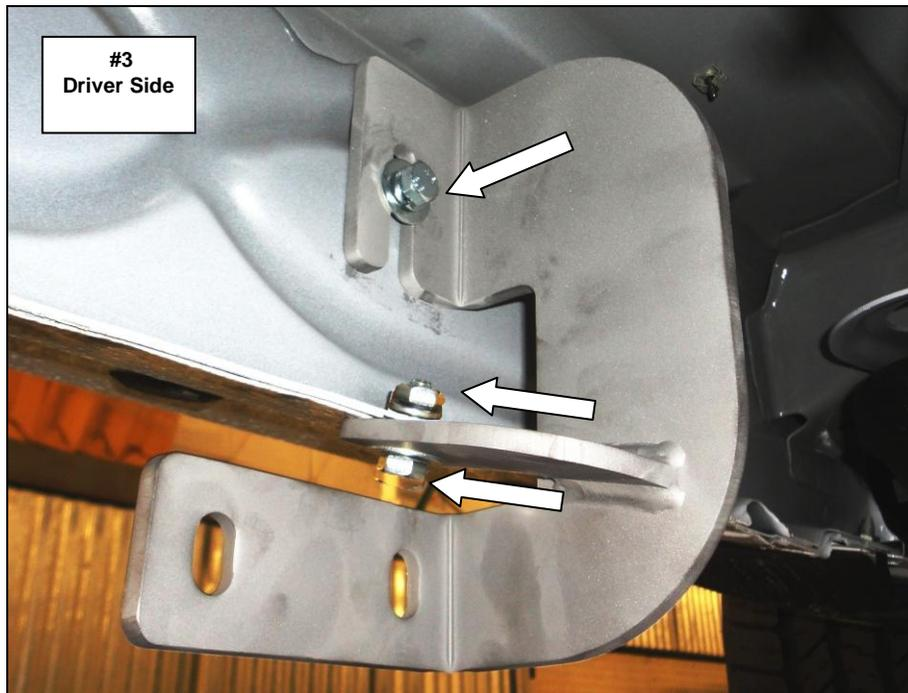
**Step-3** Install the driver side center bracket by measuring from the front fender bolt reward approximately 58 7/8" and locate the hole in the body pinch mold and the plastic plug in the rocker panel, **(Photo 4)**. Remove the plastic plug from the rocker panel and install (1) M8 U-Nut in the rocker panel, **(Photo 5)**.
