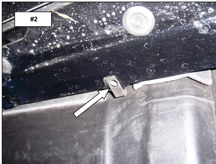
**Step-2** Locate in front of the urea tank the plastic plug in the body rocker panel. Remove the plug, Install the vinyl gasket over the threads of the 3/8" T-Bolt and install T-Bolt in the rocker panel as shown. **Photo #3 & #4**
