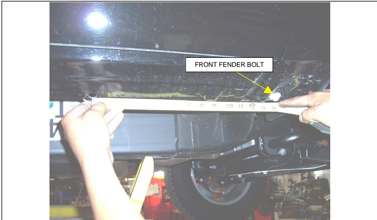
**STEP-2** This installation uses three mounting brackets per side. Begin by installing the passenger side front mounting bracket. Measure rearward from the front fender bolt approximately 14" and locate the single hole in the body pinch mold and the square nut spot welded in the rocker panel.
