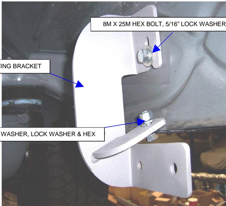
**STEP-3** Loosely attach one of the C07P mounting brackets to the rocker panel and pinch mold using the 8M, 5/16" and 3/8" fasteners as shown.
