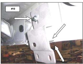
Step-6 Passenger side rear bracket installation.
