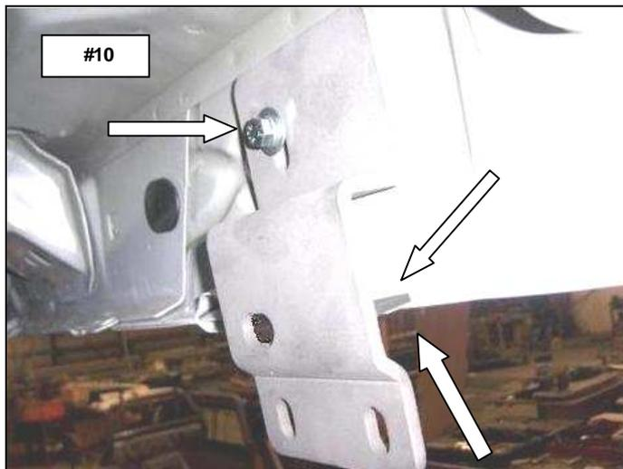
**Step-6** Passenger side rear bracket installation.
