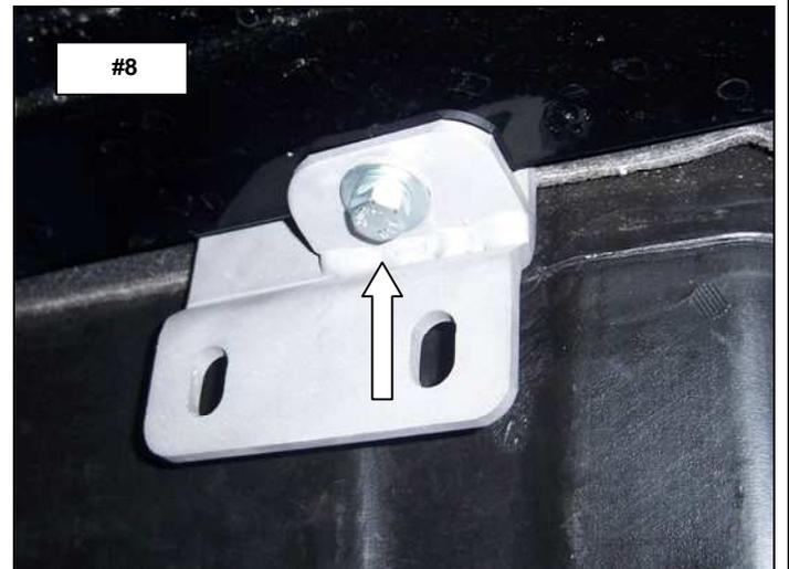
**Step-5** Passenger side Center bracket installation.
