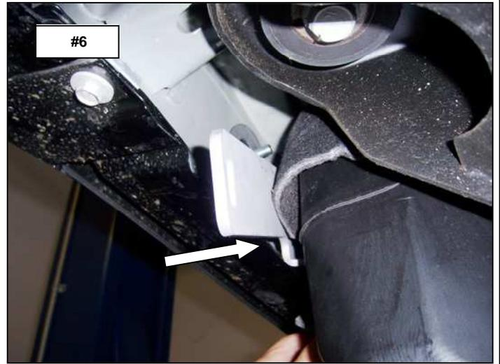
**Step-4** Position the obround hole in the front of the bracket over the T-Bolt and install (1) 3/8" flat washer, (1) 3/8" lock washer and (1) 3/8" hex nut. Position the flange of the bracket on the bottom of the pinch mold and align the obround hole with the U-Nut and install (1) 5/16" flat washer, (1) 5/16" lock washer and (1) 5/16" x 1" hex bolt. Leave the nut and bolt loose for final adjustment. **Photo #7 & #8**
