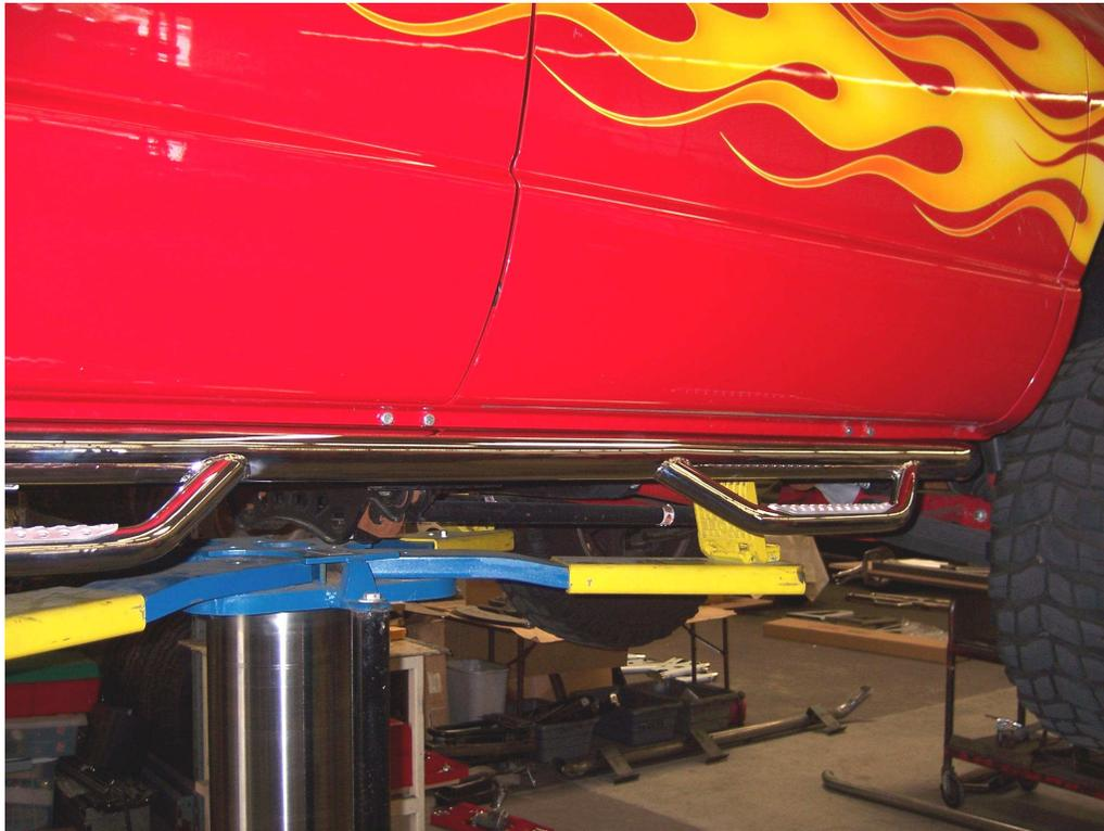
**STEP-6** Align sidestep with the body and then tighten all mounting bracket and sidestep nuts and bolts.
