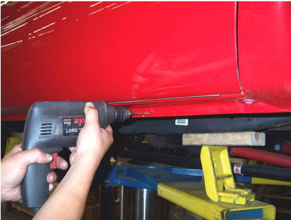
**STEP-3** Confirm the measurements, center punch and drill 3/8" holes through the body pinch mold. Repeat the above steps for the driver side.
