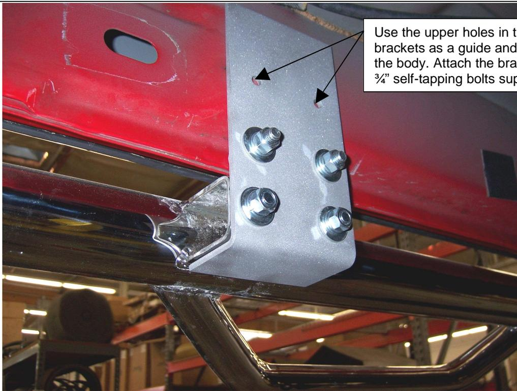
Use the upper holes in the mounting brackets as a guide and drill 3/16" holes in the body. Attach the bracket using the 1/4" x 3/4" self-tapping bolts supplied.
