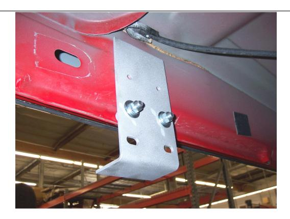
**Step 4.** Loosely attach the mounting brackets to the body pinch mold using the 3/8" x 2" hex bolts, flat washers, lock washers and hex nuts as shown.
