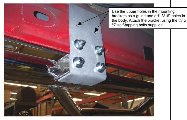
**Step 5.** Position the passenger sidestep up to the mounting brackets and loosely attach it to the brackets using the 3/8" x 1 1/4" hex bolts, flat washers, lock washers and hex nuts.
