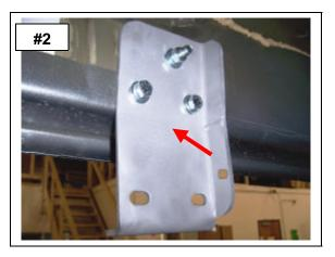
**STEP-3** LOCATE THE HEXAGON SHAPED HOLES IN THE BODY PANEL AT THE CENTER OF THE CAB AND REPEAT THE ABOVE STEPS TO INSTALL THE REMAINING CENTER BRACKET.
