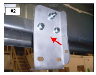
**STEP-3** LOCATE THE HEXAGON SHAPED HOLES IN THE BODY PANEL AT THE CENTER OF THE CAB AND REPEAT THE ABOVE STEPS TO INSTALL ONE OF THE D07D BRACKETS.
