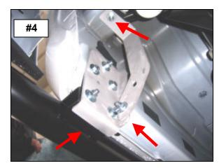
**STEP-6** ALIGN THE SIDE STEP WITH THE VEHICLE AND TIGHTEN ALL BRACKETS AND SIDE STEP NUTS AND BOLTS.
