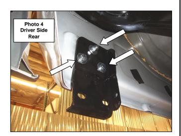
**Step-5** Locate and remove the driver side rear factory body mount bolt and washer, (**Photo 5**).
