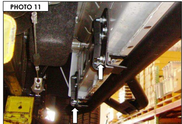
11. Align the side step with the vehicle and tighten all bracket and side step nuts and bolts. Repeat the installation steps to install the passenger side brackets and running board.
