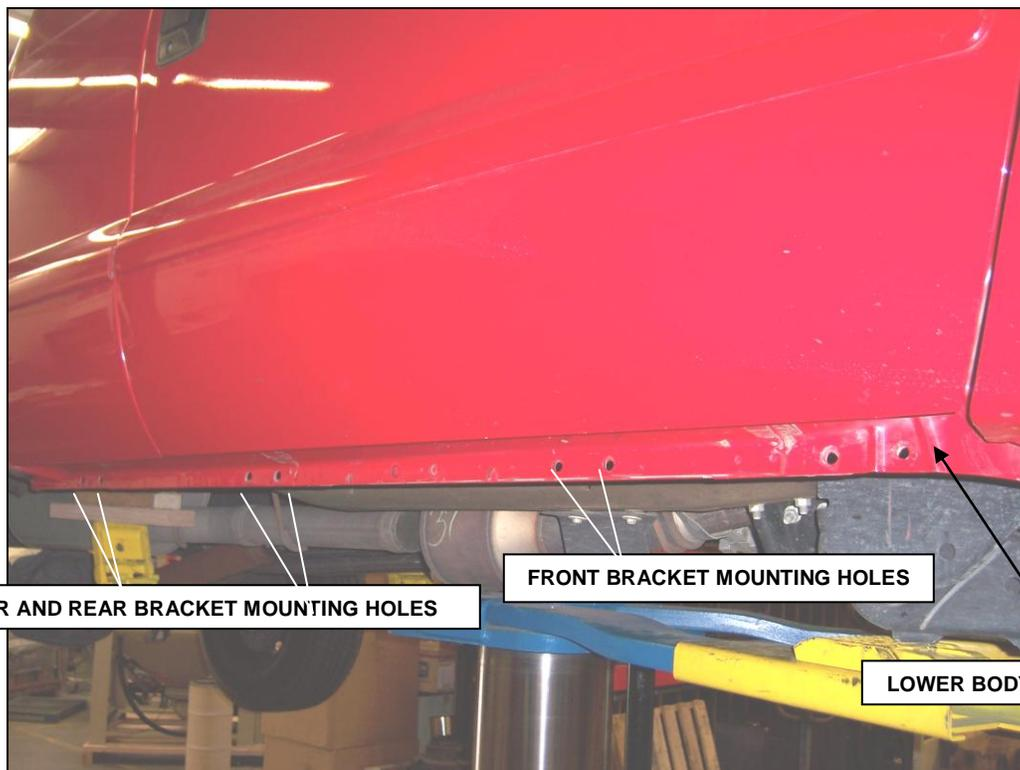
**Step-5** This installation uses three mounting brackets per side. Beginning with the passenger side, locate the holes in the rocker panel and lower body pinch mold.
