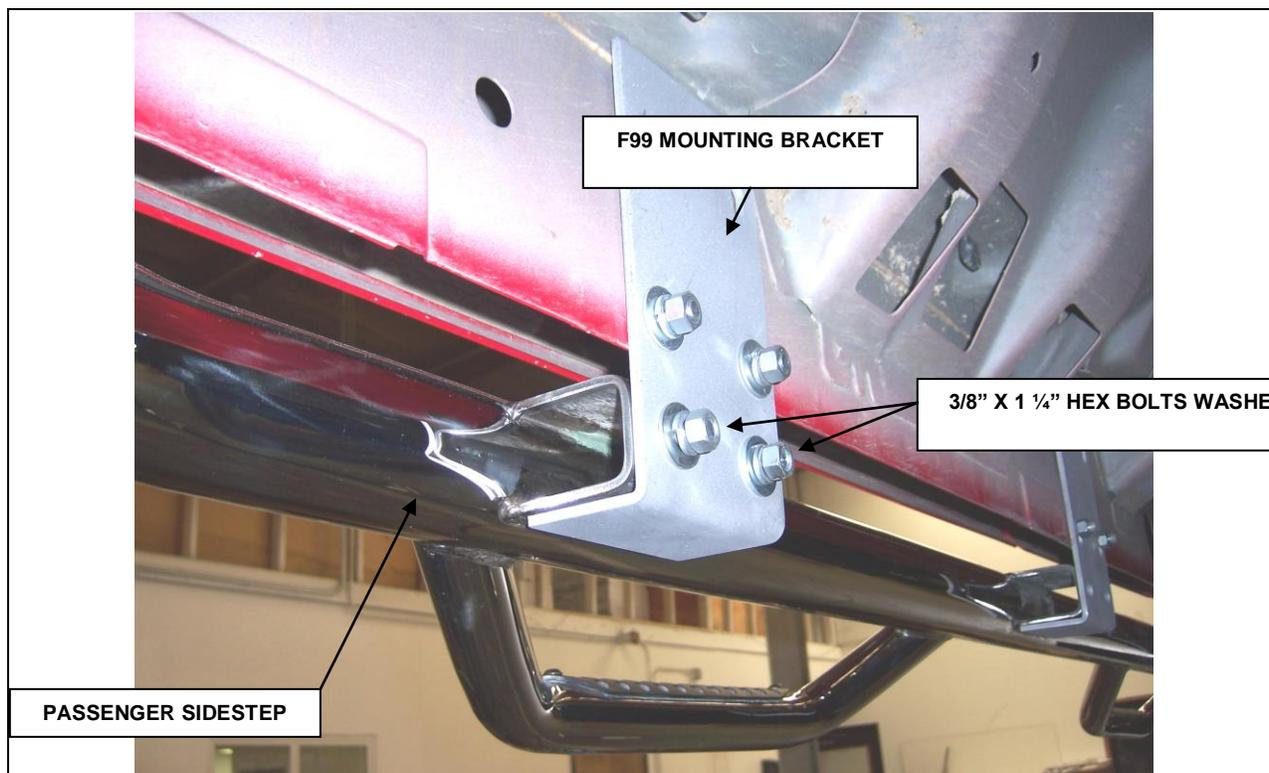
**Step-7** Position the passenger sidestep up to the mounting brackets and loosely attach it to the brackets using the 3/8" x 1 1/4" hex bolts, washers and nuts as shown.
