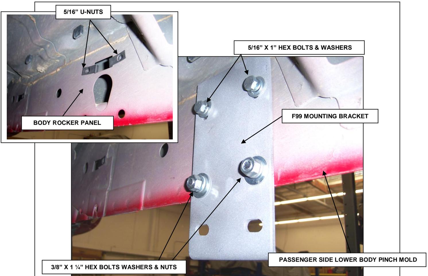
**Step-6** Install the 5/16" u-nuts in the rocker panel. Loosely attach the mounting brackets to the rocker panel and pinch mold using the 5/16" hex bolts, 3/8" hex bolts, washers, and nuts as shown.
