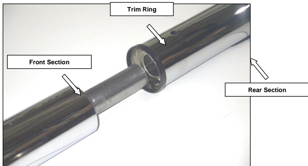
**Step-2** Insert the male end of the side step front section into the female end of the side step rear section, and position the front side step section snug against the trim ring (lip over the edge). Align the front and rear side step sections, and secure the assembly using (1) 3/8" Allen head set screw.
