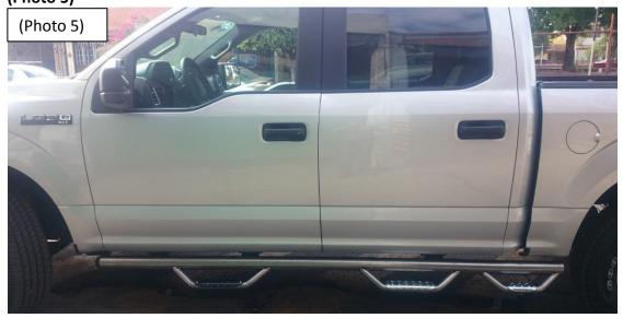
5. Repeat the above steps to install the driver side brackets and side step.
