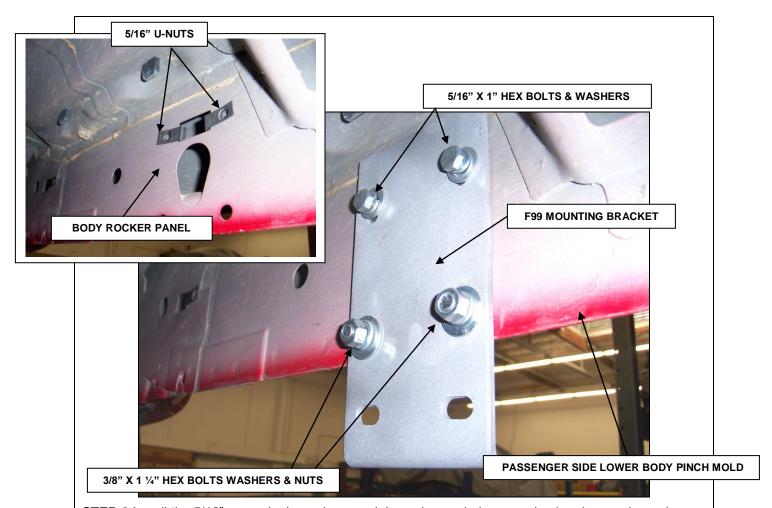
**STEP-3** Install the 5/16" u-nuts in the rocker panel. Loosely attach the mounting brackets to the rocker panel and pinch mold using the 5/16" hex bolts, 3/8" hex bolts, washers, and nuts as shown.
