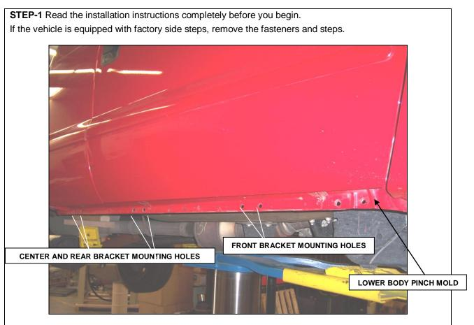
**STEP-2** This installation uses three mounting brackets per side. Beginning with the passenger side, locate the holes in the rocker panel and lower body pinch mold.
