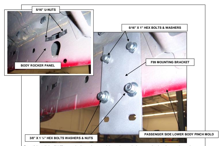
**Step-6** Install the 5/16" u-nuts in the rocker panel. Loosely attach the mounting brackets to the rocker panel and pinch mold using the 5/16" hex bolts, 3/8" hex bolts, washers, and nuts as shown.
