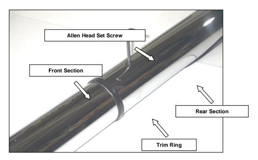
**Step-3** Install the plastic plug in the set screw access hole to conceal the set screw.
