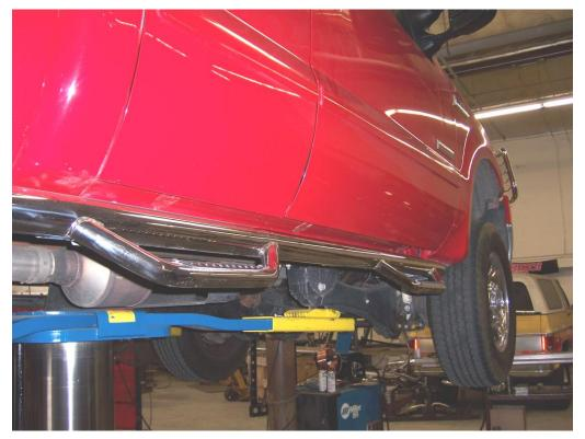
**Step-8** Align sidestep with the body, and then tighten all mounting bracket and sidestep nuts and bolts. Repeat the above steps to install the driver side mounting brackets and sidestep.
