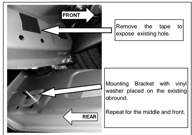
5.- To attach the front and middle bracket, attach to the bolt on the mounting bracket that went in by vehicle panel with: 3/8" flat and lock washer, 3/8" hex nut. And the nut on the mounting bracket with: 3/8 x 1" hex head bolt, 3/8" flat and lock washer. **SEE ILLUSTRATION 2.** Leave loose.
