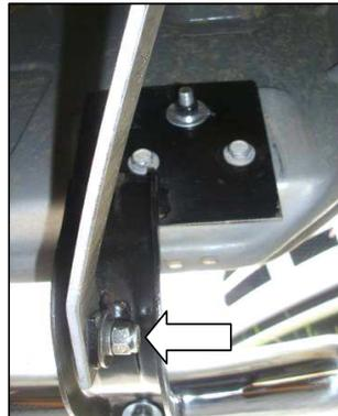
Rear auxiliary bracket installed on bracket.
