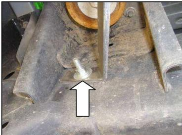
Rear auxiliary bracket installed on chassis.
