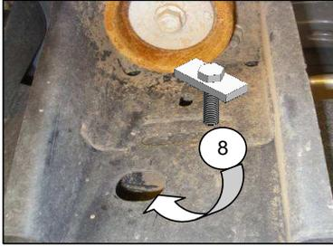
Insert the 3/8" bolt plate in hole indicated.
