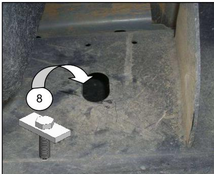
Insert the 3/8" bolt plate in hole indicated.
