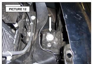
10. Attach the Grille Guard FS to the top of the upper brackets using the  $1/2 \times 1 \ 1/2$ " carriage bolts, 1/2" flat washers, 1/2" lock washers and 1/2" hex nut and to the outside of the lower brackets using the  $1/2 \times 1 \ 1/2$ " hex bolts, 1/2" flat washers, 1/2" lock washers and 1/2" hex nut. Align the Grille Guard FS with the vehicle and tighten all nuts and bolts. **See pictures 13 and 14.**
