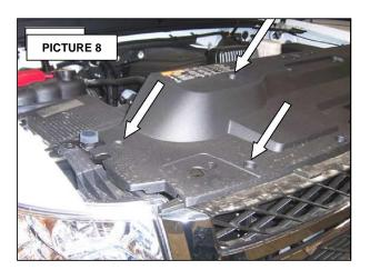
7. Remove the screws securing the top of the grille. Seer picture 9.
