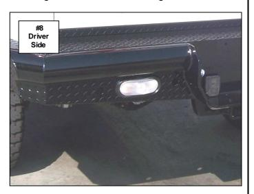
**Step-8** Align the replacement bumper with the vehicle, verify that the tailgate clears when lowered, and tighten all nuts and bolts. If necessary, loosen the nuts and bolts to adjust the bumper. Remember to check and retighten the nuts and bolts periodically.
