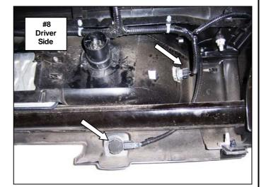
**Step-5** Remove the trailer plug from the factory bumper, install it to the replacement bumper, and reconnect the wiring harness. **Picture #7**
