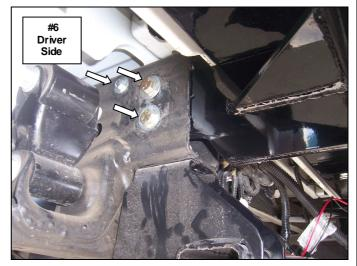
**Step-3** The center of the replacement bumper will sit directly on top of the receiver hitch. Secure the replacement bumper to the receiver hitch using (2)  $\frac{1}{2}$ " hex bots, (2)  $\frac{1}{2}$ " flat washers and (2)  $\frac{1}{2}$ " flange nuts. Leave the nuts and bolts loose for final adjustment. **Picture #7**
