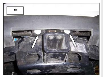
**Step-5** Remove the bolts (1) per side securing the bumper brackets and receiver hitch to the bottom of the frame using 21mm socket and ratchet. **Picture #3**
