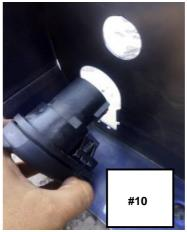
**Step 5-** Install the license plate lights in the replacement bumper. The license plate lights are self-grounding; you will only need to connect a hot wire to each light. Use a circuit tester to find the hot wire from the factory license plate light wiring, and then splice the red wire from the provided lights to the hot wire. Note: It may be necessary to scuff the paint around the backside of the holes in the replacement bumper to make a good connection with the light housing.
