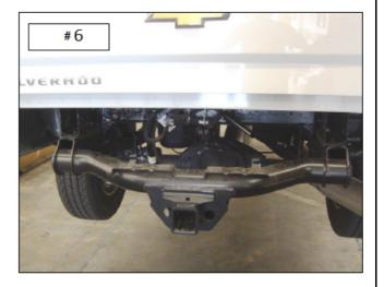
Step- 9 Remove the license plate, disconnect the license plate lights, and If equipped disconnect the backup sensors from the factory bumper wiring harness.
