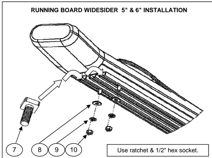
9. If you acquired a Oval side bar widesider 4", place on brackets and attach with: 5/16" square head bolt, 5/16" Flat and lock washer. **SEE ILLUSTRATION 7.** Repeat for the opposite side. Leave loose.
