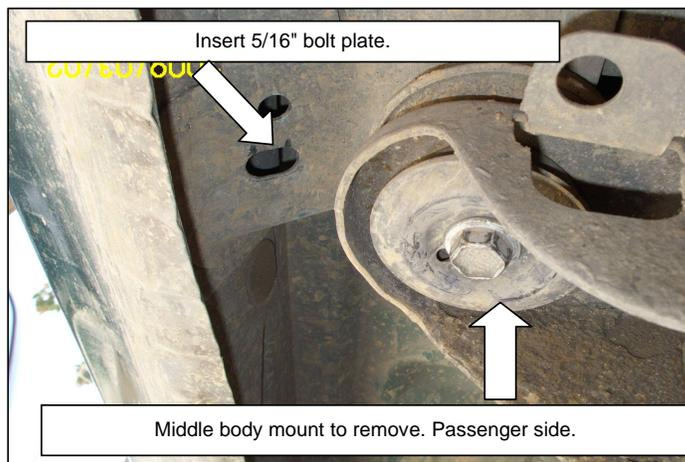
5. Install the middle bracket and attach with bolts before removed. Locates the hole that is in the rocker panel of the vehicle and inserts 5/16" bolt plate. Mounts the middle auxiliary bracket and attach with: 5/16" flat and lock washers, 5/16" hex nut. In the other side of the bracket attach with the middle bracket: 3/8 x 1" carriage head bolt, 3/8" flat and lock washers, 3/8" hex nut. **SEE PICTURE 2, ILLUSTRATION 4.** Leave loose.
