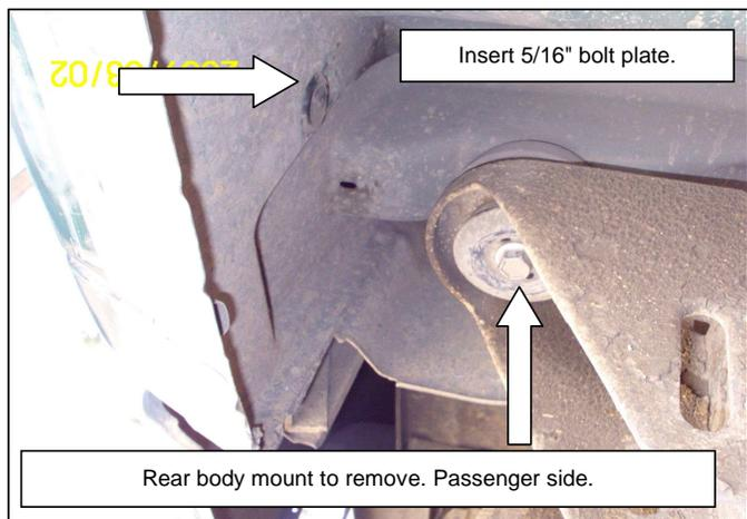
7. Install the middle bracket and attach with bolts before removed. Locates to the rubber plug that is in the rocker panel of the vehicle, remove and insert 5/16" bolt plate.
