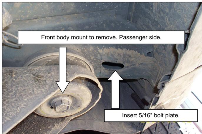
3. Install the front bracket and attach with bolts before removed. Locates the hole that is in the rocker panel of the vehicle and inserts 5/16" bolt plate. Mounts the front auxiliary bracket and attach with: 5/16" flat and lock washers, 5/16" hex nut. In the other side of the bracket attach with the front bracket: 3/8 x 1" carriage head bolt, 3/8" flat and lock washers, 3/8" hex nut. **SEE PICTURE 1, ILLUSTRATION 3.** Leave loose.
