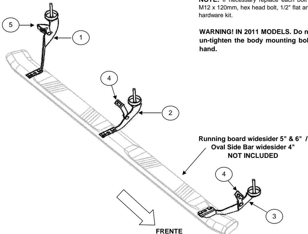
**NOTE:** If necessary replace each bolt that holds the body mount by: M12 x 120mm, hex head bolt, 1/2" flat and lock washers, including in the hardware kit.
