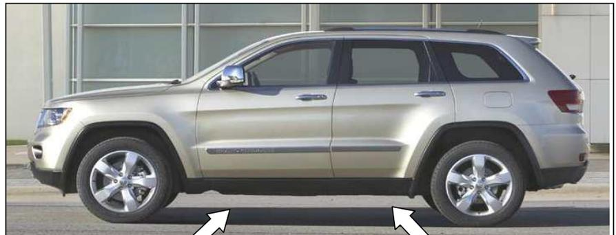
Under this part in the body install the front bracket, driver side shown.
