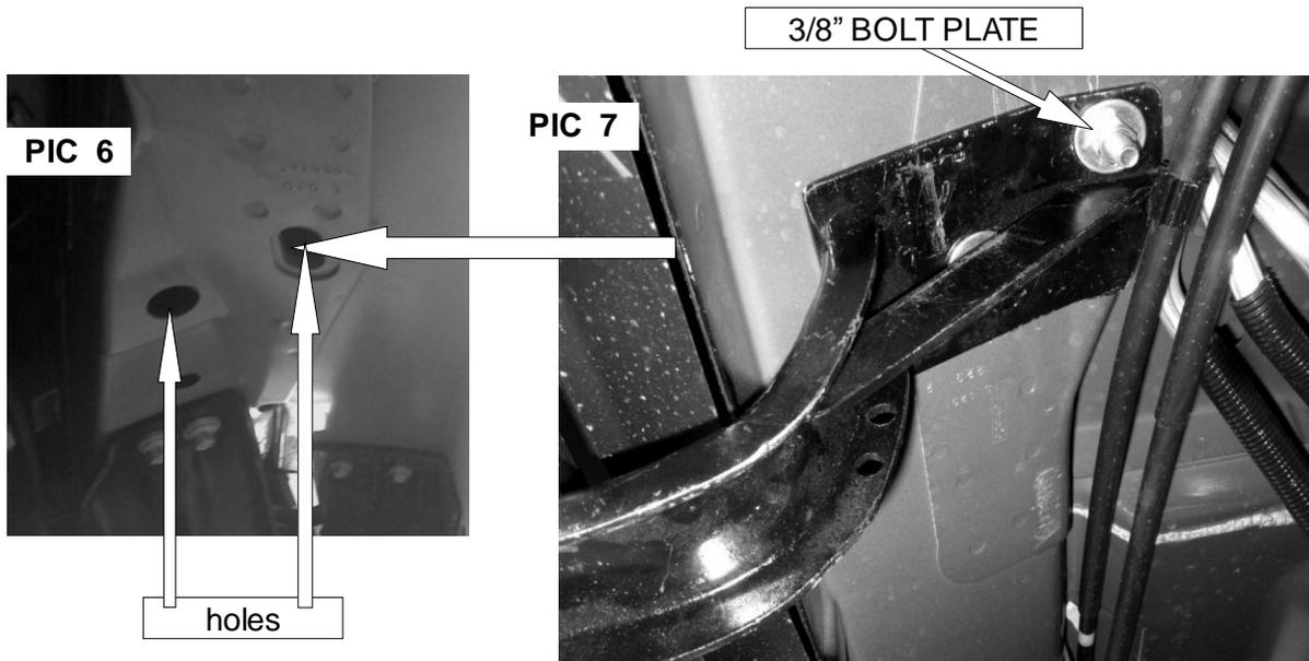
7. Place the side bar on the installed brackets and attach whit "U" bracket from the side bar hardware kit. Attach whit 5/16" square head bolts, 5/16" flat and lock black washers. ( PIC 8)
