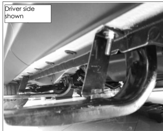
12. To install the rear bracket, locate the existing obround in the rear of the rocker panel **(see picture 7)** and insert a 1/2" bolt plate. Attach the rear bracket to the 1/2" bolt plate using (1) flat washer, (1) lock washer and (1) hex nut 1/2". Attach the other end of the auxiliary rear bracket to the rear bracket with (1) hex bolt 5/16 x 1", (1) flat washer, (1) lock washer and (1) hex nut 5/16". **(See picture 8).** Do not tighten. Repeat this procedure to install the passenger side.
