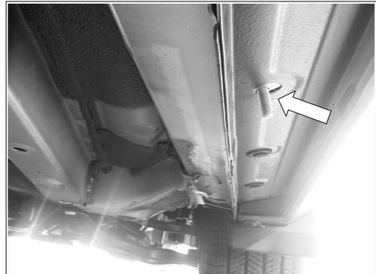
15. To install the passenger's front bracket, locate in the rail two existing holes, one of them is covered with a rubber plug, remove it. Thread the 3/8" bolt guide to the 3/8" round bar bolt then insert the tip of the guide into the hole shown in picture 10 until tip appears through the other hole. Pull the bolt guide until the threads of the bolt extends out through the rail. Picture 11.
