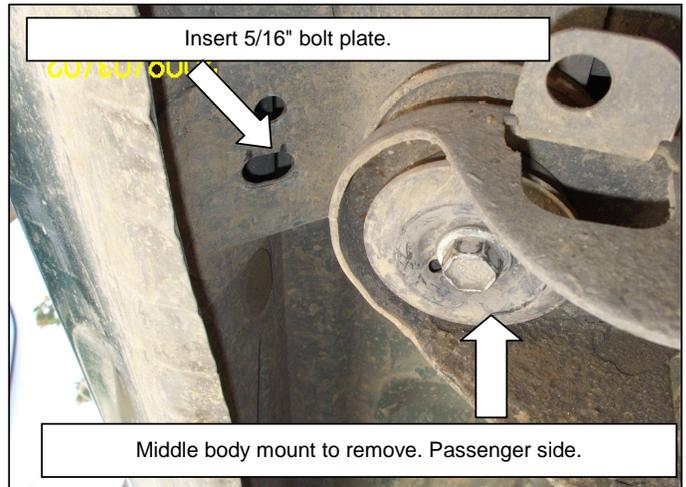
5. Install the middle bracket and attach with bolts before removed. Locates the hole that is in the rocker of the vehicle and inserts 5/16" bolt plate.
