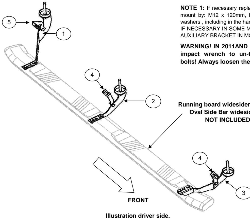
**NOTE 1:** If necessary replace each bolt that holds the body mount by: M12 x 120mm, hex head bolt, 1/2" flat and lock washers, including in the hardware kit.
