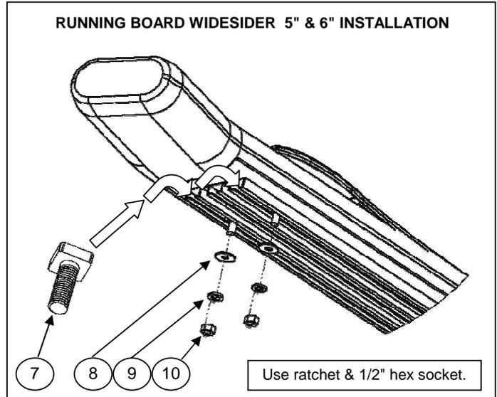
9. If you acquired a Oval side bar widesider 4", place on brackets and attach with: 5/16" square head bolt, 5/16" Flat and lock washer. **SEE ILLUSTRATION 7.** Repeat for the opposite side. Leave loose.
