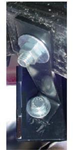
Auxiliary mounting bracket passenger side
