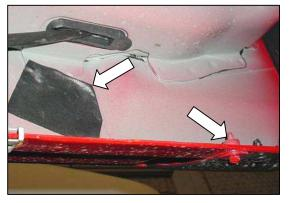
Remove this cover hole tape and bolt & clip nut. Front driver's side shown.
