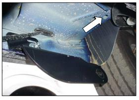
Insert into the square hole steel bar with 5/16" bolt. Front driver's side shown.
