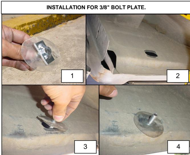
3. Place (1) front mounting bracket attach to the 3/8" bolt plate previously placed using: 3/8" flat and lock washers and 3/8" hex nut. Leave loose.
