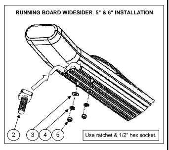
5. If you acquired a Oval side bar widesider 4", place on brackets and attach with: 5/16" square head bolt, 5/16" Flat and lock washer.
