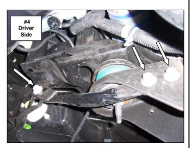
**Step-5** Remove the nut and bolts' securing each of the tow hooks to the frame using an 18mm wrench, socket, and ratchet. **Picture #5**
