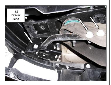
**Step-4** Remove the nut and bolts' securing each of the tow hooks to the frame using an 18mm wrench, socket, and ratchet. **Picture #3**
