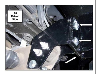
**Step-3** Install the auxiliary brackets by positioning the shorter offset end inside the frame and the opposite end on top of the bracket welded to the lower tube of the replacement bumper. Align the holes and secure the auxiliary bracket to the frame using (1)  $\frac{1}{2}$ " x 1  $\frac{1}{2}$ " hex bolt, (1)  $\frac{1}{2}$ " flat washer and (1)  $\frac{1}{2}$ " flange nut. **Picture #7**
