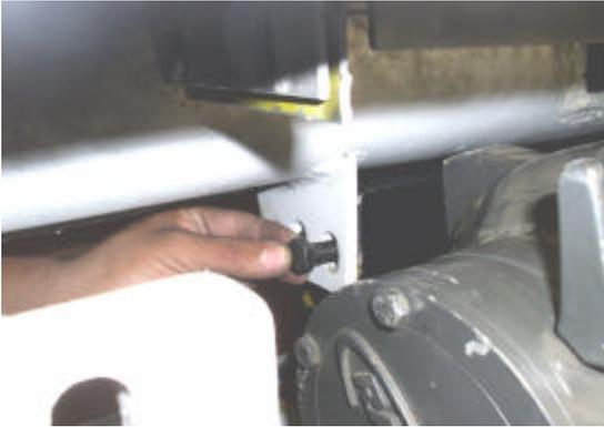
10. Align winch tray's holes with upper bracket's holes; attach using ( 4 ) 1/2 x 1 1/2" hex head bolts with 1/2" lock washers. Leave loose. **Picture 5.**
