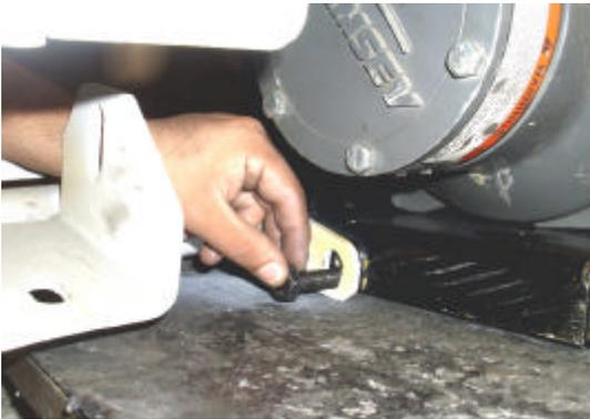
11. Align winch tray's holes with lower bracket's holes; attach using ( 4 ) 1/2 x 1 1/2" hex head bolts with 1/2" lock washers. Leave loose. **Picture 6.**
