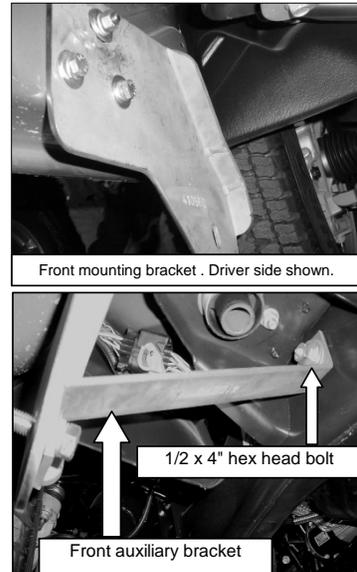
4. To install auxiliary rear mounting bracket, locate existing hole in the chassis support. **See Picture 3.** Introduce (1) 3/8 x 1 1/4" hex head bolt then place rear auxiliary mounting bracket and secure to the bolt previously placed using (1) 3/8" flat and lock washers and 3/8" hex nut. Secure the other end to the rear mounting bracket using (1) 3/8 x 1 1/4" hex head bolt, (1) 3/8" flat and lock washers and (1) 3/8" hex nut. Leave loose. **Picture 4.**
