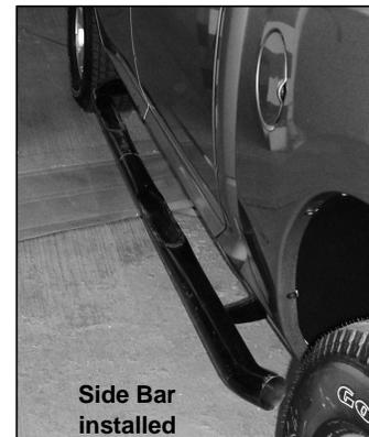
6. Align the Side Bar to the vehicle and tighten all hardware. Finally place a plastic plug into the hole of the tube's joint.
