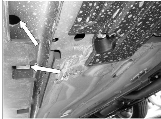
6. Place and attach the front bracket to the 3/8" bolt plates using (1) 3/8" flat washer, (1) 3/8" lock washer and (1) 3/8" hex nut by each bolt. Leave loose. Picture 3.
