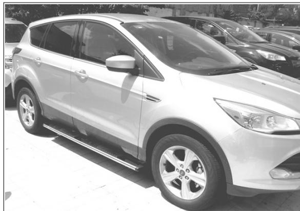
the widesider with the vehicle and tighten the mounting brackets and square bolts. Repeat the installation steps to install the driver side brackets and widesider. Remember to periodically check and retighten all nuts and bolts.
