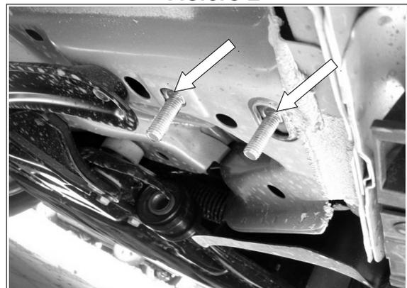
4.- Beginning with the passenger side. Locate underneath the vehicle at front and rear of the platform the bracket's fixation points. Picture 1.
