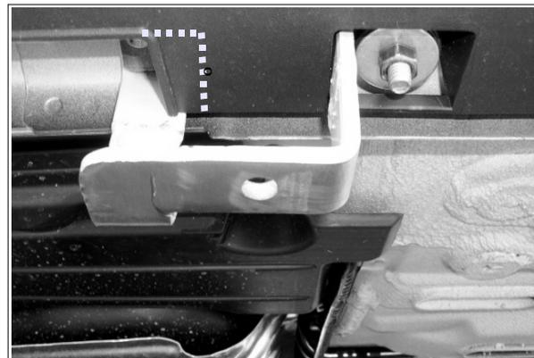
8. Locate the existing hole behind the auxiliary rear bracket. Insert a 3/8" bolt plate then place the rear bracket and secure using (1) 3/8" flat and lock washers and (1) 3/8" hex nut. Picture 7.
