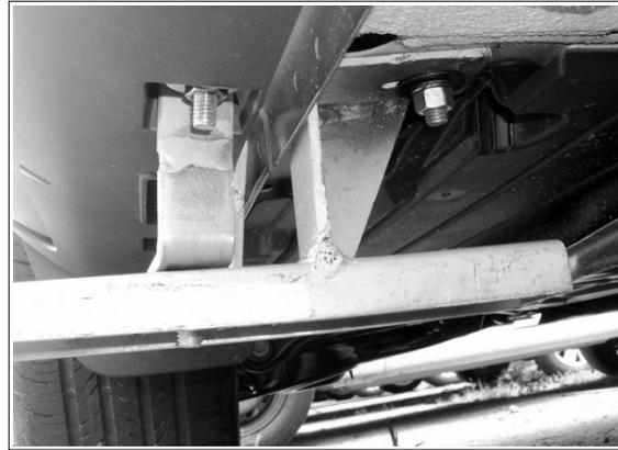
9. Secure auxiliary rear bracket to the rear bracket with (1) 3/8" x 1" hex bolt, (1) 3/8" flat and lock washers, and (1) 3/8" hex nut. Picture 8.
